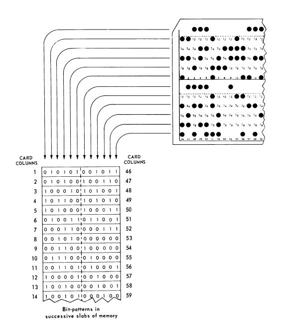
FEED a Punched Card and READ Columns READ Columns from a Punched Card 400 card per minute reader (90 columns)
